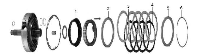
**Installation:** Stack the Overdrive clutch pack as follows; install modified apply piston (1), install return spring and retaining bolts, install the bottom .192" apply plate (2), install friction (3), install Kolene® steel plate (4), You will be alternating friction and steel plates, 5 frictions and 4 steel plates, install top .192" pressure plate (5) and snap ring (6)
